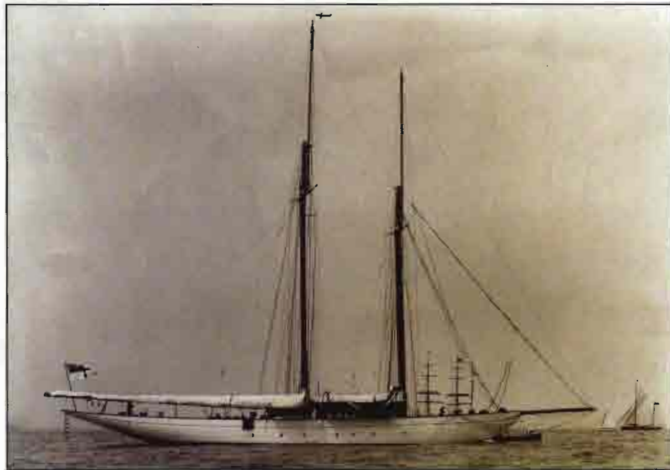
As Sylvana , the future Orion moored in the Solent in 1911. The large central coachroof covers a beautiful saloon, still preserved as it was; notice also the size of the topmasts, the boom and the bowsprit.
