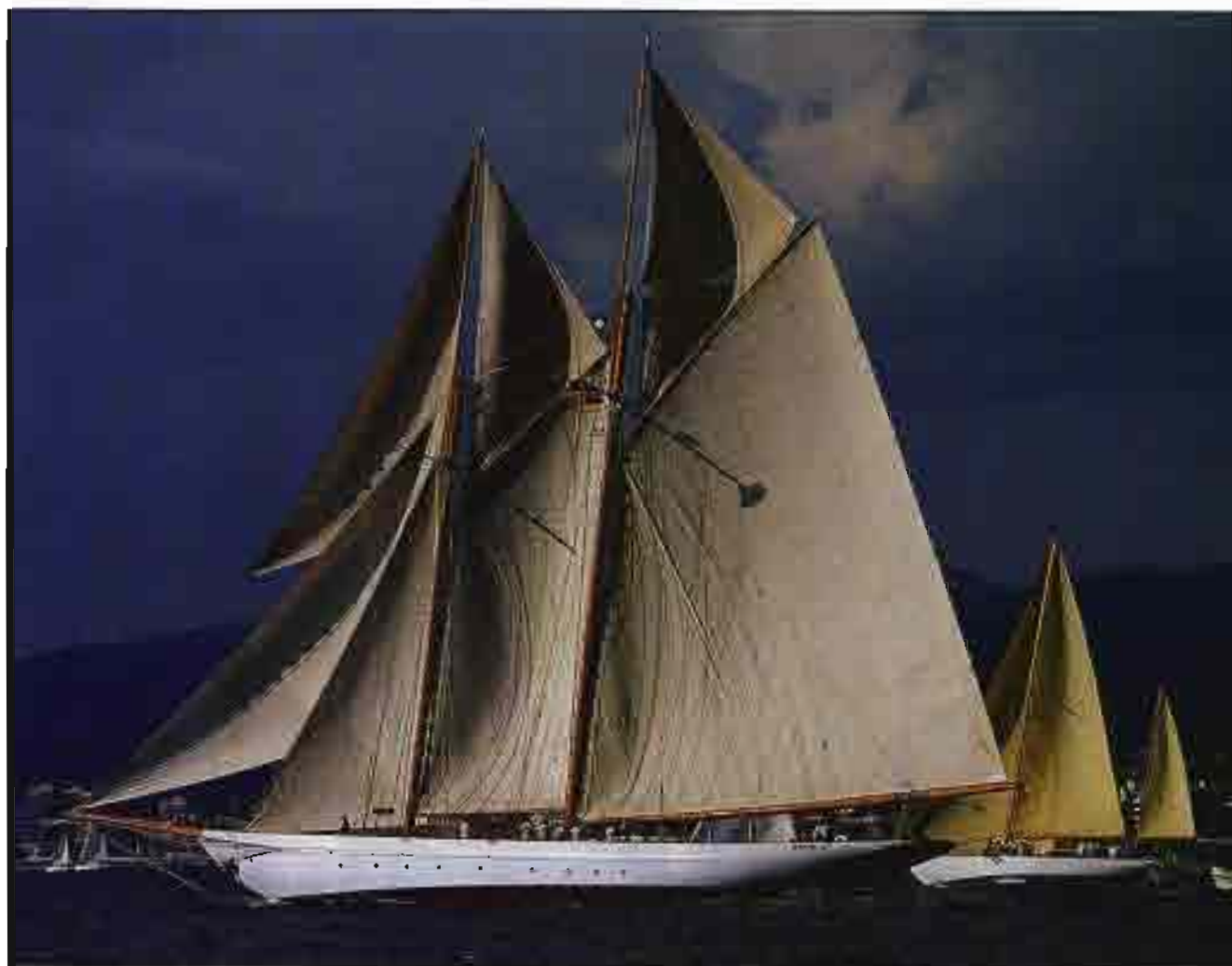
The current rig resembles the 1910 rig in design, except that the masts are very slightly shorter. But the bowsprit and boom have been restored to their original length.
