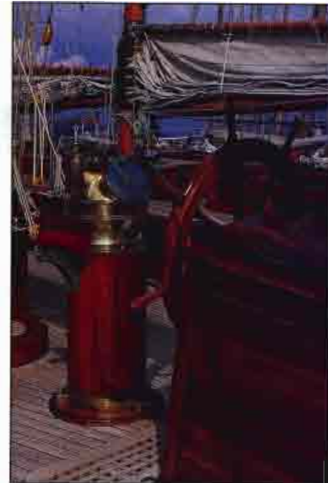
The compass column mounted on the brass binnacle; the helmsman stands on the wheel side.
